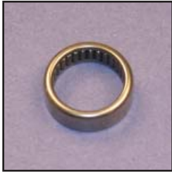
BEARING # 928 SAGINAW INPUT SHAFT (23.3MM X 28.5MM X 9.3MM)
